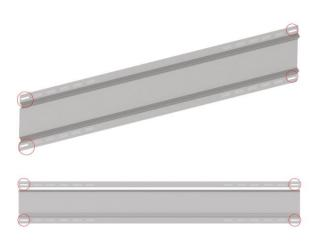
3. Use a flat-bladed screwdriver to break out of the holes in the shield that overlap with the holes of the UPG...MC holders from point 2.
