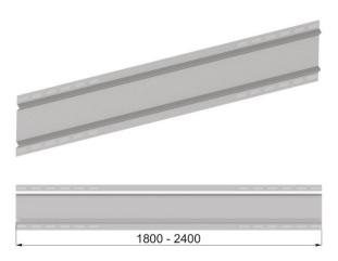
1. The length of the shields is selected based on: panel length + 60 mm
